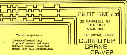
The CRANE CONTROLLER provides a simple method of connecting a model crane to the B.B.C. micro. The control unit has relay outputs to control the directions of three motors one at a time. In addition a switch circuit is connected for controlling lights, horns or an electro-magnet for picking up objects.
